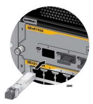
Figure 90. Installing an SFP+ Transceiver in the AT-SBx81XS6 Line Card
