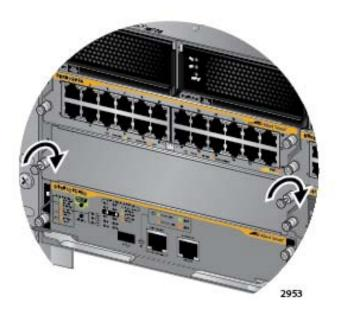
Figure 79. Tightening the Thumbscrews on a Blank Slot Cover
