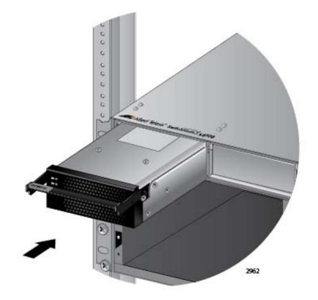
Figure 57. Inserting the AT-SBxPWRPOE1 Power Supply
