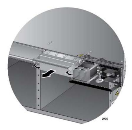
Figure 59. Removing the Blank Slot Cover from Power Supply Slot C
