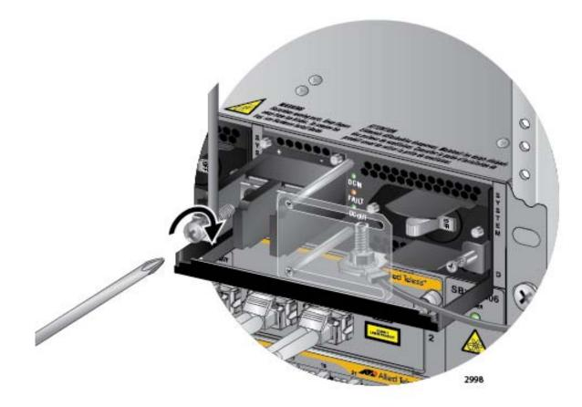
Figure 130. Connecting the Positive Lead Wire
