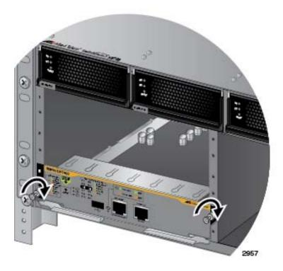
Figure 73. Tightening the Thumb Screws on the AT-SBx81CFC400 Card
