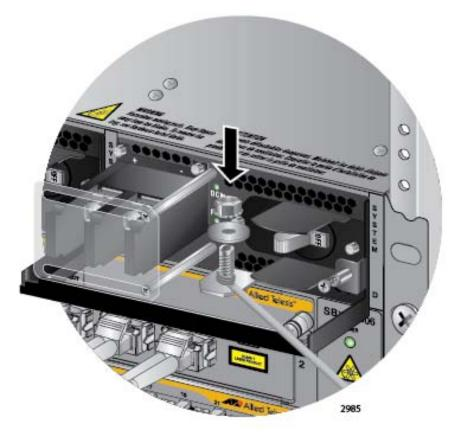
Figure 111. Securing the Bare Grounding Wire to the Grounding Post
