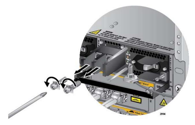
Figure 125. Removing the Terminal Screws
