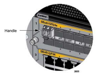
Figure 86. Verifying the Position of the Handle on the SFP Transceiver on the AT-SBx81GS24a Line Card
