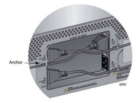
Figure 101. Securing the Power Cord for the AT-SBxPWRPOE1 Power Supply to an Anchor
