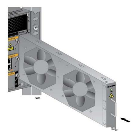
Figure 157. Installing a New AT-SBxFAN06 Fan Module
