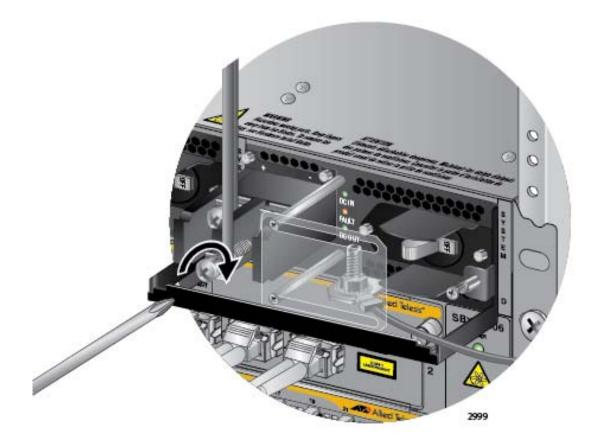
Figure 131. Connecting the Negative Lead Wire
