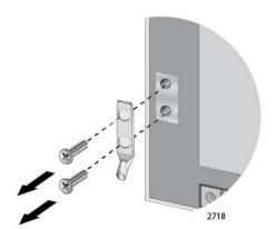
Figure 42. Removing the Grounding Lug
