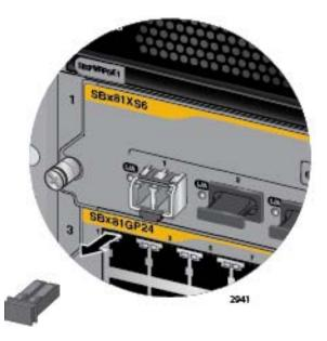
Figure 91. Removing the Dust Cover from an SFP+ Transceiver in the AT-SBx81XS6 Line Card
