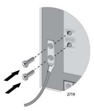
Figure 44. Installing the Grounding Lug and Wire
