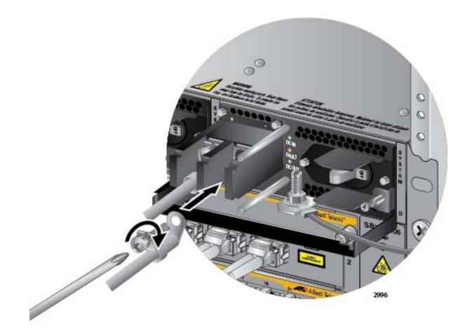
Figure 127. Connecting the Negative (-) Power Wire with a Right Angle Terminal
