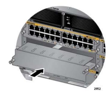
1. Position a blank slot cover over an unused slot, as shown in Figure 78.
