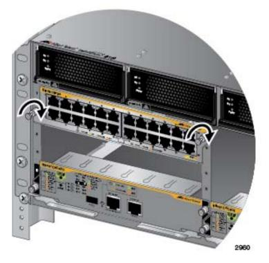
Figure 77. Tightening the Thumb Screws on an Ethernet Line Card
