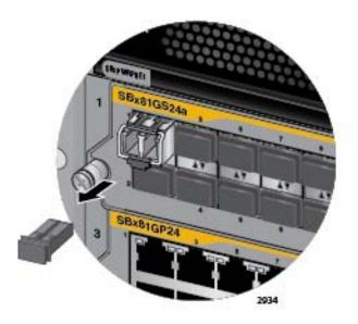
Figure 85. Removing the Dust Cover from the SFP Transceiver in the AT-SBx81GS24a Line Card
