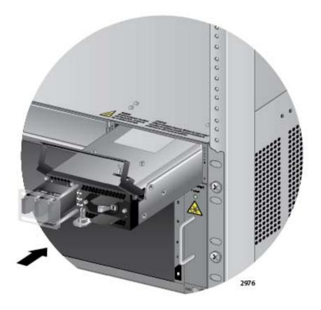
Figure 63. Inserting the AT-SBxPWRSYS1 DC Power Supply
