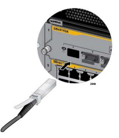
Figure 96. Installing the AT-SP10TW Cable in the AT-SBx81XS6 Line Card
