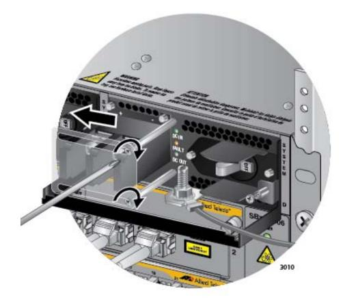
Figure 147. Closing the Plastic Cover
