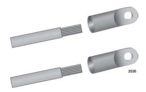
Figure 114. Attaching the Power Wires to the Straight Terminal Lugs
