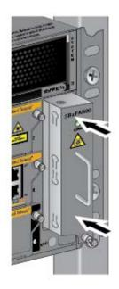
Figure 158. Securing the AT-SBxFAN06 Fan Module on the Backplane Connector
