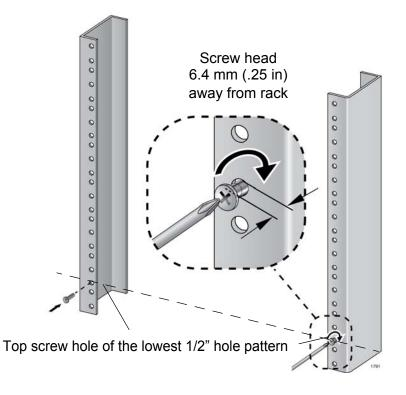
Figure 30. Rack Mounting Hole Locations
