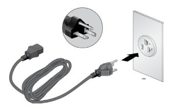
Figure 28. 100 - 125 VAC 125 V NEMA 5-20 Plug and Receptacle
