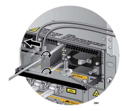
Figure 120. Closing the Plastic Cover over the Terminal Connectors
