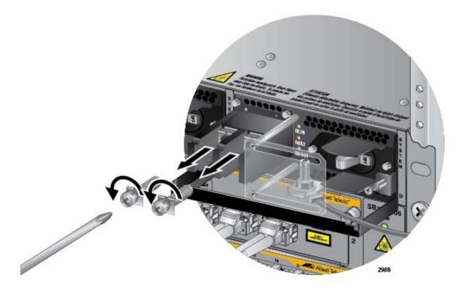
Figure 117. Removing the Terminal Screws
