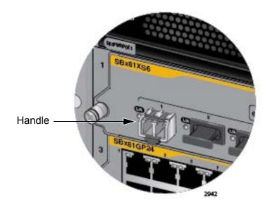
Figure 92. Verifying the Position of the Handle on the SFP+ Transceiver on the AT-SBx81XS6 Line Card
