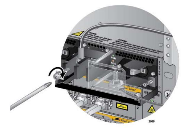
Figure 118. Connecting the Positive (+) Power Wire with a Straight Terminal
