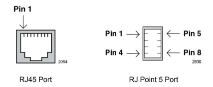
Figure 160. Pin Numbers for RJ-45 and RJ Point 5 Ports (Front View)
