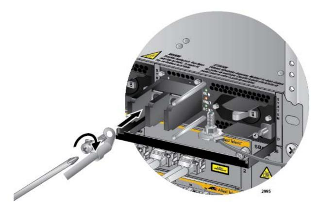
Figure 126. Connecting the Positive (+) Power Wire with a Right Angle Terminal
