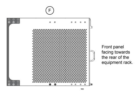
Figure 36. Rack Bracket Locations for Reverse Position of Chassis
