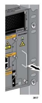
Figure 154. Loosening the AT-SBxFAN06 Fan Module from the Backplane Connector
