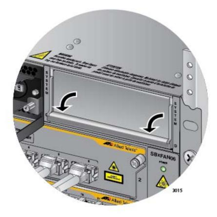
Figure 152. Lowering the Locking Handle on the Power Supply Slot Cover
