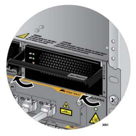
Figure 138. Lifting the Locking Handle on the Power Supply
