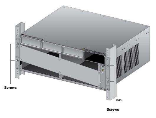
Figure 38. Installing the Rack Mount Screws
