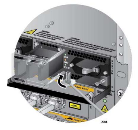
Figure 110. Attaching the Bare Grounding Wire to the Grounding Post
