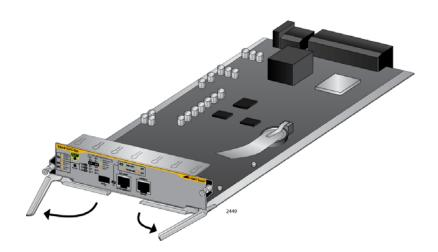
Figure 69. Opening the Locking Handles on the AT-SBx81CFC400 Controller Fabric Card
