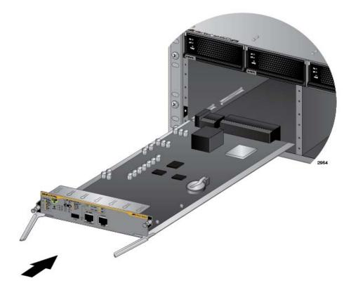
Figure 71. Aligning the AT-SBx81CFC400 Card in the Chassis Slot
