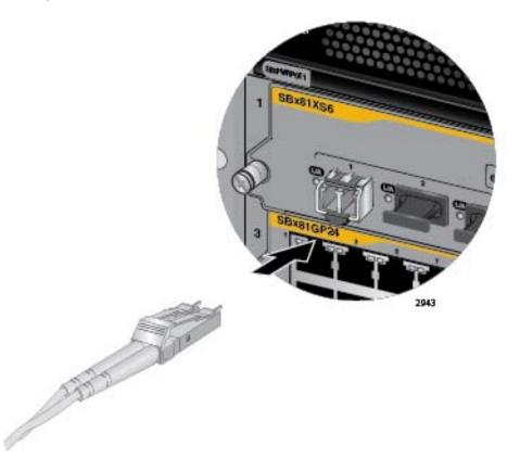
Figure 93. Attaching a Fiber Optic Cable to an SFP+ Transceiver in the AT-SBx81XS6 Line Card
