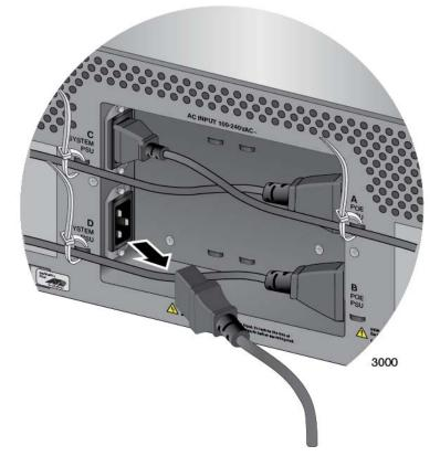
Figure 137. Disconnecting the AC Power Cord from the AC Socket on the Back Panel
