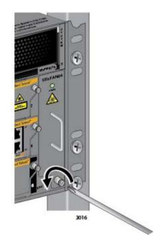
Figure 153. Loosening the Screw on the AT-SBxFAN06 Fan Module
