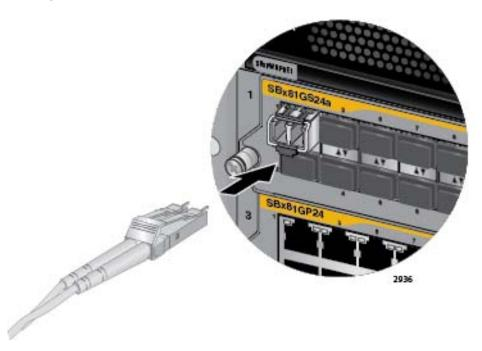
Figure 87. Attaching a Fiber Optic Cable to an SFP Transceiver in the AT-SBx81GS24a Line Card
