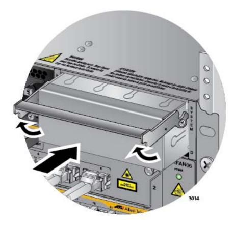
Figure 151. Installing a Blank Power Supply Slot Cover
