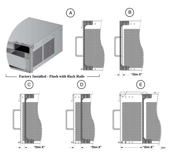
Figure 35. Rack Mounting Bracket Locations
