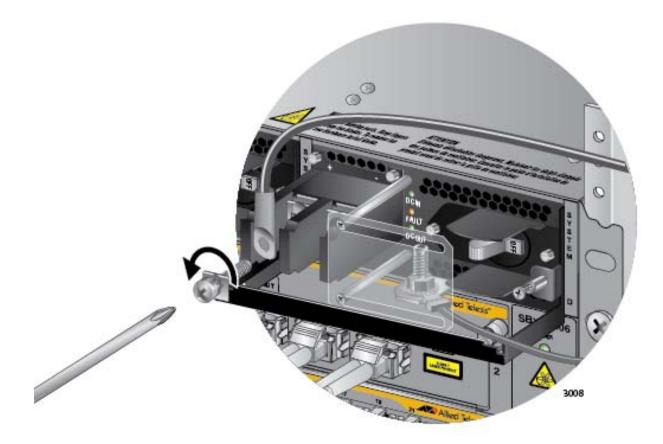
Figure 145. Removing the Positive Lead Wire from the Terminal Block
