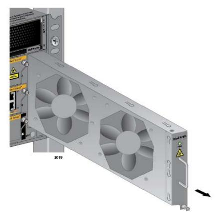
Figure 156. Removing the AT-SBxFAN06 Fan Module from the Chassis
