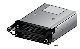
Figure 56. Unlocking the Handle on the AT-SBxPWRPOE1 Power Supply
