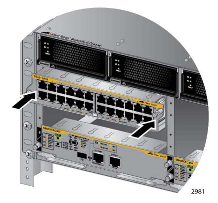
Figure 76. Seating an Ethernet Line Card on the Backplane Connector
