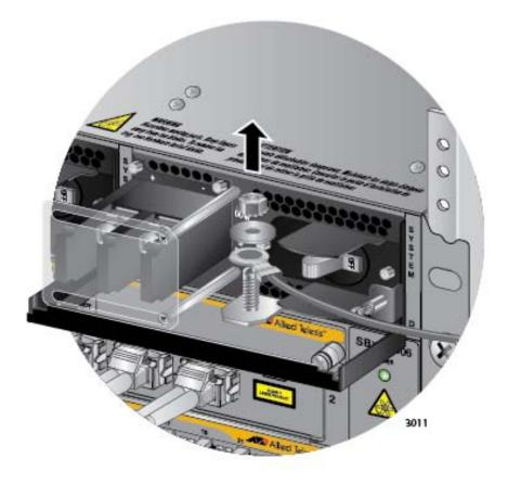
Figure 148. Removing the Grounding Wire
