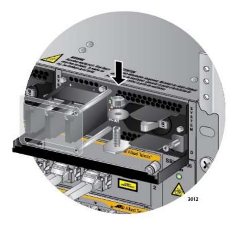
Figure 149. Reinstalling the Nut and Washer on the Grounding Post
