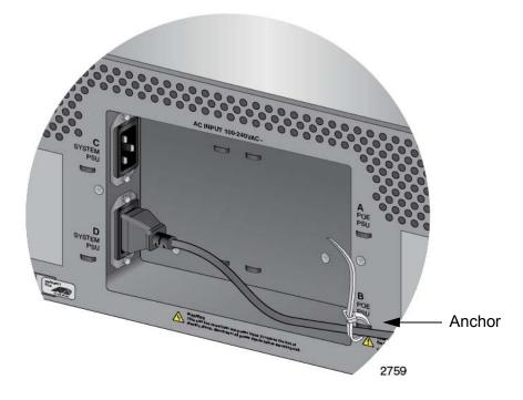
Figure 99. Securing the Power Cord for the AT-SBxPWRSYS1 AC Power Supply to an Anchor
