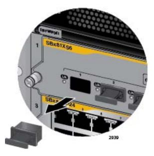
Figure 88. Removing the Dust Cover from an SFP+ Slot in the AT-SBx81XS6 Line Card
