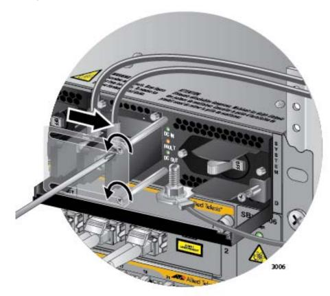
Figure 143. Opening the Plastic Window on the Terminal Block
