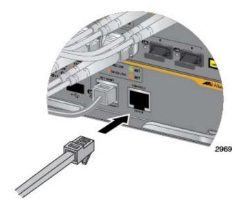
Figure 134. Connecting the Management Cable to the Console RS-232 Port
