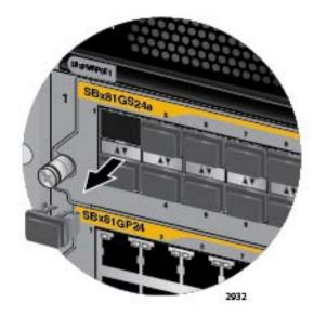
Figure 82. Removing the Dust Cover from an SFP Slot in the AT-SBx81GS24a Line Card 3. To install the transceiver in an SFP slot on the top row of the line card, orient the transceiver with the handle on top, as shown in Figure 83. To install it into a slot on the bottom row of the line card, orient it with the handle on the bottom.
