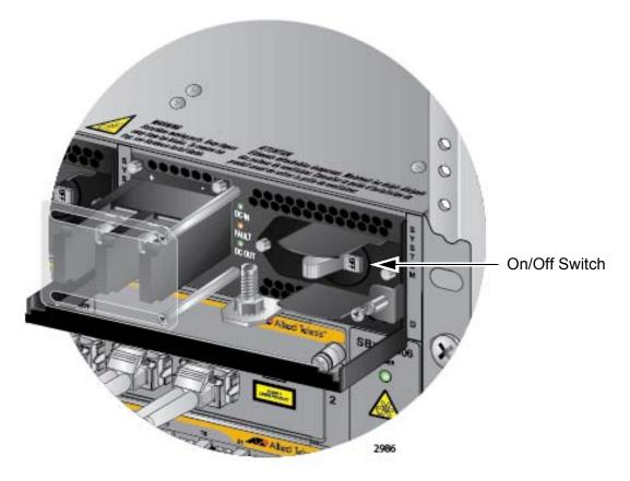
Figure 115. On/Off Switch on the AT-SBxPWRSYS1 DC Power Supply
