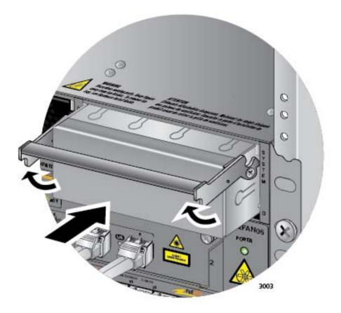
Figure 140. Installing a Blank Power Supply Slot Cover
