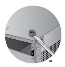
Figure 34. Removing the Rubber Feet
