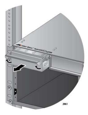
Figure 53. Removing the Blank Slot Cover from Power Supply Slot A
