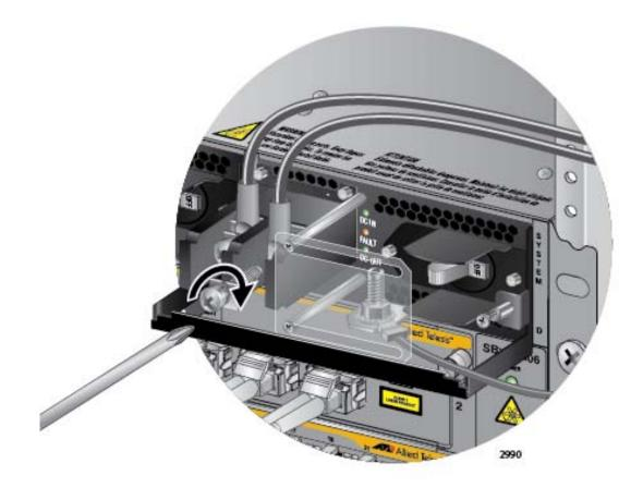
Figure 119. Connecting the Negative (-) Power Wire with a Straight Terminal
