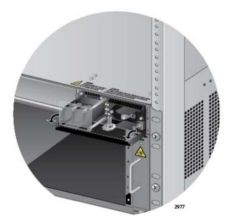
Figure 64. Locking the Handle on the AT-SBxPWRSYS1 Power Supply
