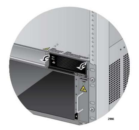
Figure 52. Lowering the Handle on the AT-SBxPWRSYS1 Power Supply
