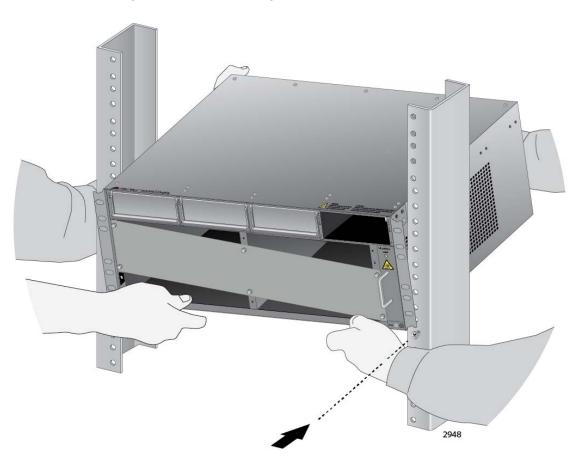
Figure 37. Lifting the AT-SBx8106 Chassis into the Equipment Rack
