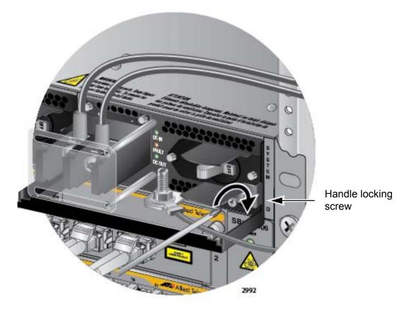
Figure 121. Tightening the Handle Locking Screw
