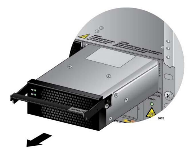
Figure 139. Removing the Power Supply from the Chassis
