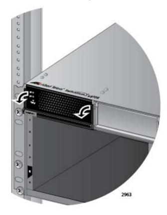
7. Lower the locking handle of the power supply module to secure the module in the slot, as shown in Figure 58.
