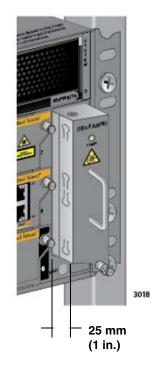
Figure 155. Withdrawing the AT-SBxFAN06 Fan Module 25 mm (1 in.) from the Chassis
