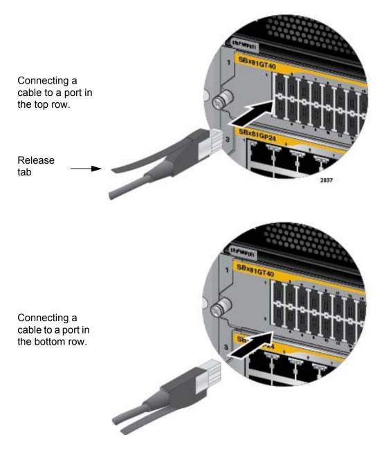
Figure 81. Connecting Cables to Ports on the AT-SBx81GT40 Line Card
