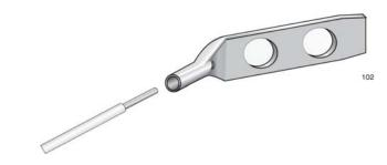
Figure 43. Attaching the Grounding Wire to the Grounding Lug
