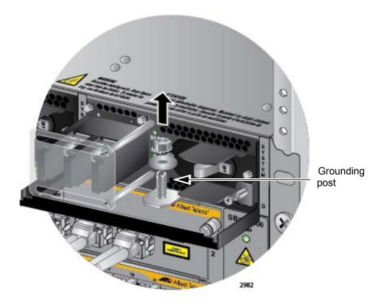
Figure 107. Removing the Nut and Washer from the Grounding Post
