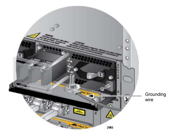
Figure 108. Installing the Grounding Wire
