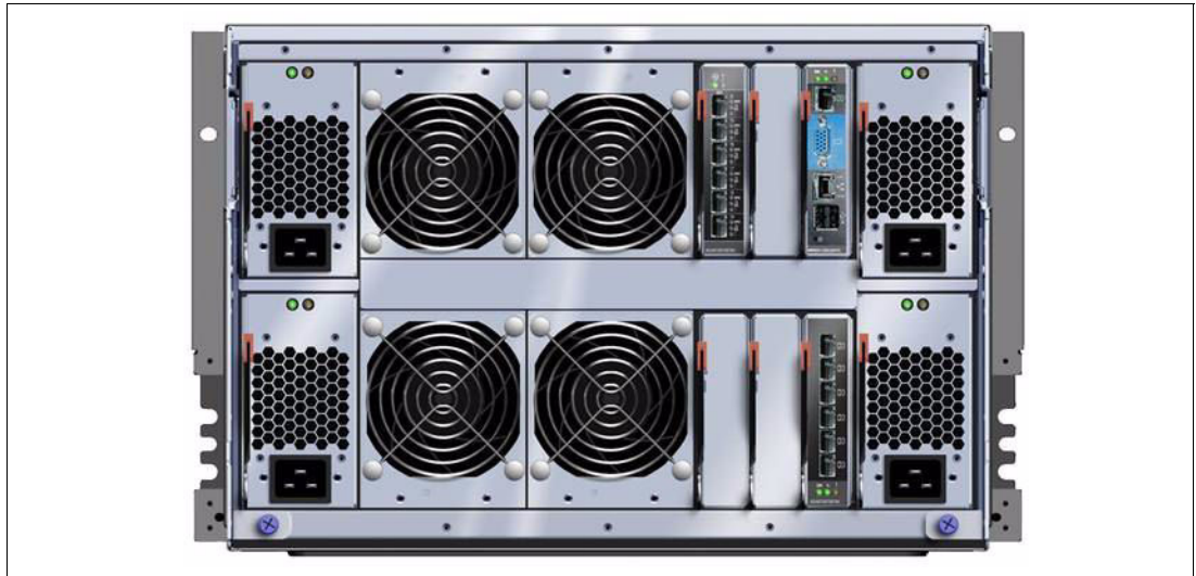
Figure 1-9 The rear of the BladeCenter S chassis
