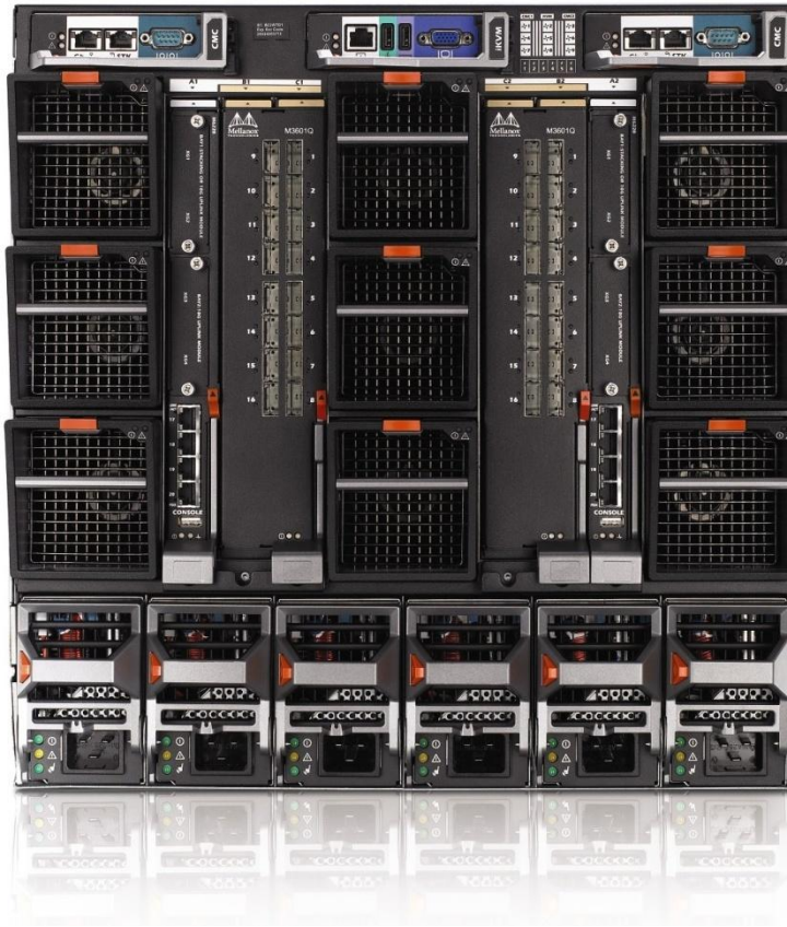
Figure 10. Rear View Showing Fans
