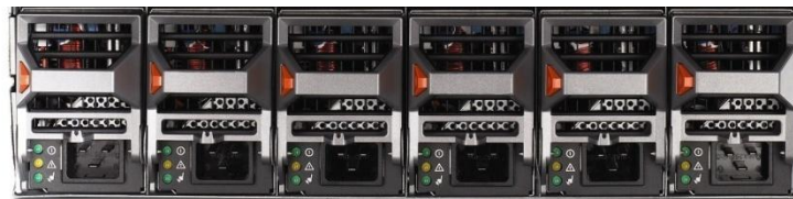
Figure 21. Power Supplies in M1000e
