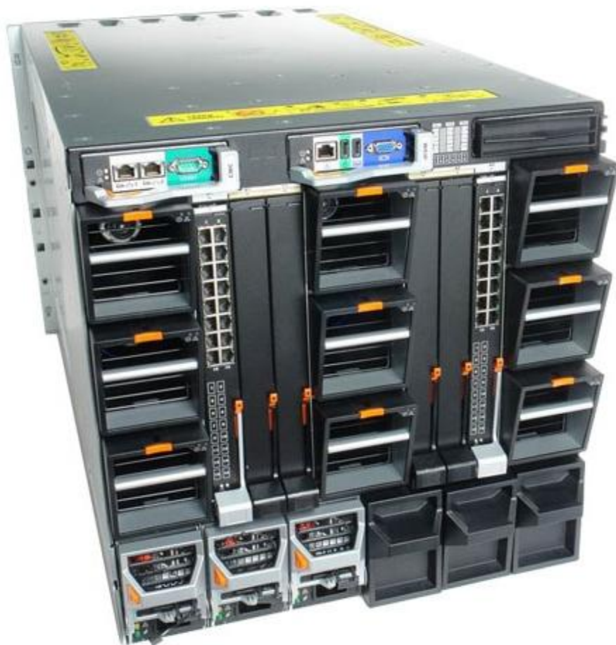
Figure 14. Installed CMC, I/O Module, and Power Supply Blanks
