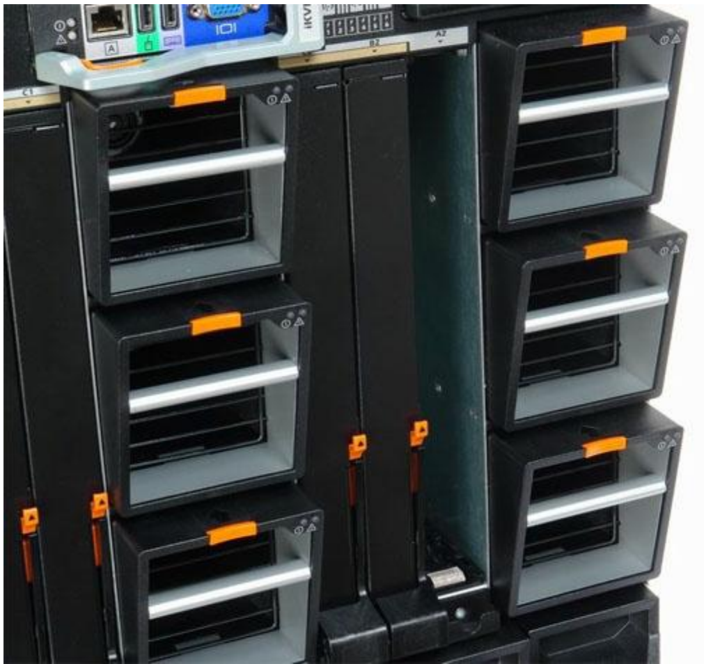
Figure 13. I/O Module and Open Slot Needing to be Filled
