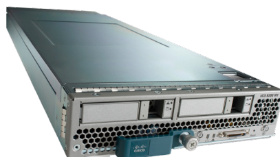
Figure 1: Cisco UCS B200 M1 Blade Server
