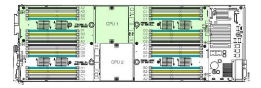
Each channel pair is identified by a letter: A, B, C, or D for each CPU. Each DIMM pair member is identified by numbers, 0, 1, 2 or 3. Additional DIMMs must be installed as shown in Table 2.
