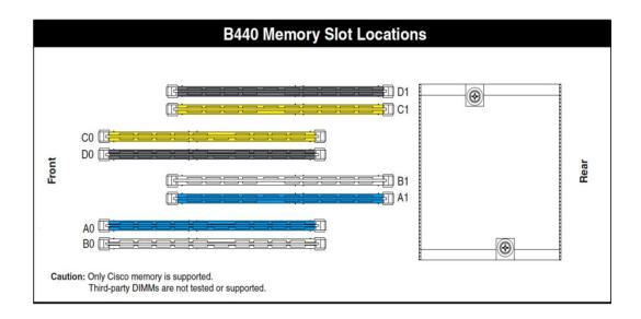
Additional DIMMs must be installed in pairs, as laid out in Table 3. The slots inside the brackets are electrically paired with each other, and should be populated with identical matched DIMMs that were ordered as a pair. Do not swap a paired DIMM with a DIMM that is not identical in manufacturer part number.
