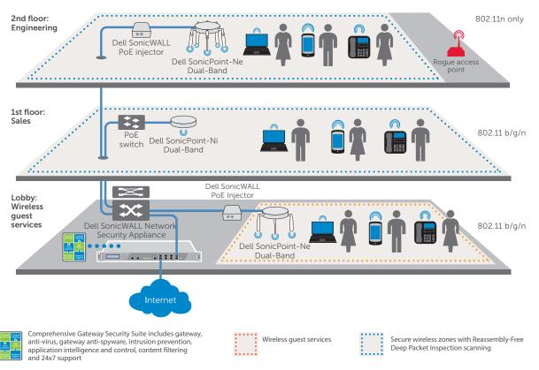
In distributed organizations, SonicPoint-N Series wireless access points automatically contact Dell SonicWALL firewalls to auto-provision the latest firmware and configurations, easing rapid deployment. Dell SonicWALL firewalls offer a single point of wireless monitoring and management, lowering total cost of infrastructure ownership. The SonicPoint-N Series provides built-in wireless Intrusion Detection Systems (IDS) to scan for rogue access points and prevent unauthorized access.
