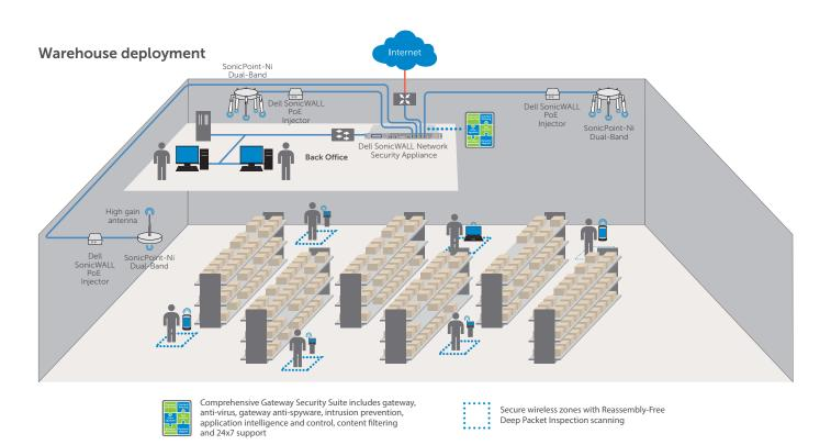
In warehouse deployments, SonicPoint-N Series wireless access points automatically contact a Dell SonicWALL firewall to auto-provision the latest firmware and configurations, simplifying rapid wireless deployment. Dell SonicWALL firewalls offer a single point of wireless monitoring and management, lowering total cost of infrastructure ownership. SonicPoint-Ni Dual-Band and SonicPoint-Ne Dual-Band come with built-in wireless IDS to scan for rogue access points and prevent unauthorized access.
