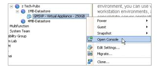
When the console window opens, click inside the window, type snwlcli at the login: prompt and then press Enter. Your mouse pointer disappears when you click in the console window. To release it, press Ctrl+Alt.
