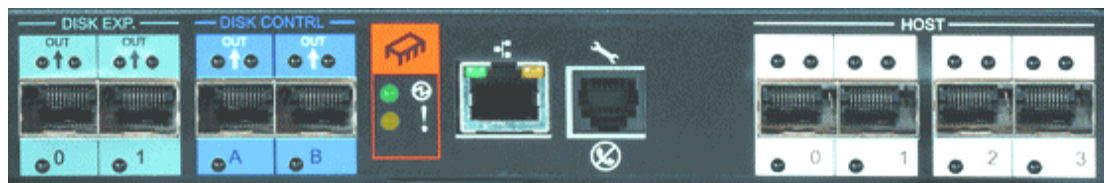
Figure 2-15 DS6800 controller card
