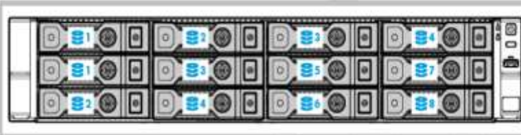
12-bay LFF hot-plug drive model
