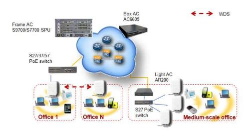
In this network , the AP7130DN-AC functions as a Fit AP and provides only data forwarding functions. The AC is responsible
