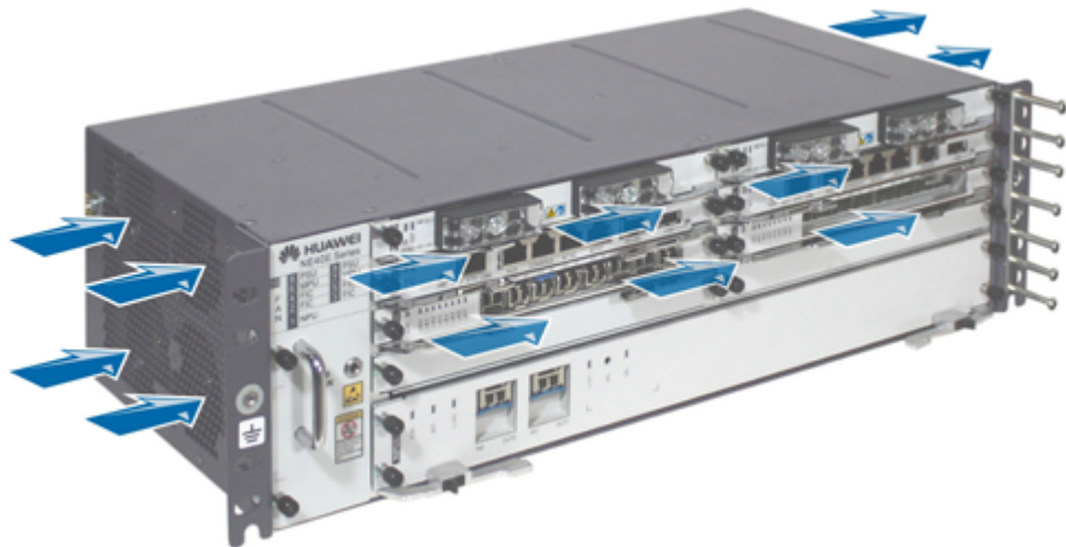
Figure 1-8 Air flow in the NE40E-X1
