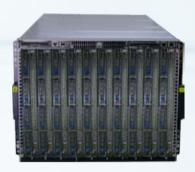
The E6000 chassis is 8U high and features an optimized layout structure to maximally use space. It houses 10 server blades and redundant PSUs, fan modules, management modules, and switch modules. The E6000 chassis can be installed in a standard 19-inch rack at a depth of at least 1000 mm. Two types of E6000 chassis are provided: AC and DC.
