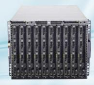
The E6000H chassis adopts the optimized layout and space design from the E6000 chassis, and uses a high-speed and passive backplane to support 8G FC or 10GE switching, making it an excellent choice for high-density and clustered deployment scenarios. The E6000H chassis can be installed in a standard 19-inch rack at a depth of at least 1000 mm. Two types of E6000H chassis are provided: AC and DC.
