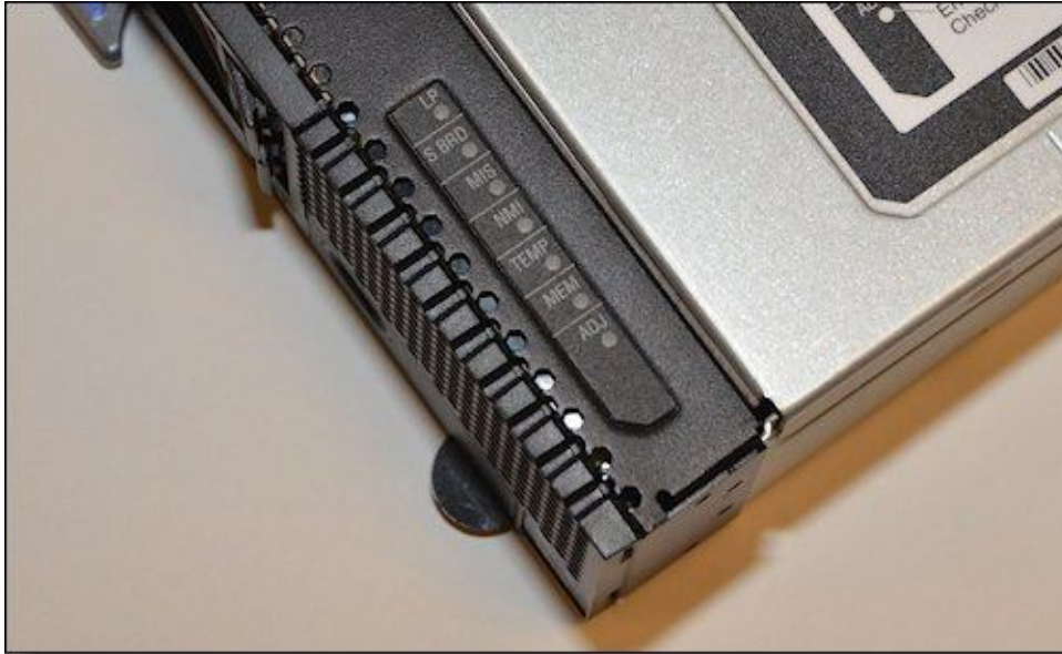
Figure 9. Location of x220 light path diagnostics panel
