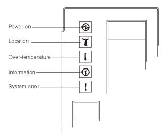
View the system LEDs remotely through the advanced management module Web interface. The main LED page shows the external LEDs on the chassis panels and the front panel. The internal blade LEDs are also available through a blade hyperlink from the LED page. This enables you to see the status of the internal LEDs on the blade server without having to turn off the blade server, remove it from the chassis, and activate the light path indications.
