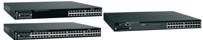
IBM b-type y-series Ethernet switches are offered in 24-port and 48-port stackable models for robust growth
