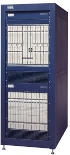
The BPX 8680 builds upon proven Cisco ATM technology that forms the backbone in the world's largest data networks and shares technology with the MGX 8800 to scale to the industry's highest port densities. The BPX 8680 consists of one or more MGX 8850s connected as feeders to a BPX 8620. Architected for very large installations, the BPX 8680 can scale to 16,000 DS1s by adding up to 16 MGX 8850 concentrator shelves while still being managed as a single node.
