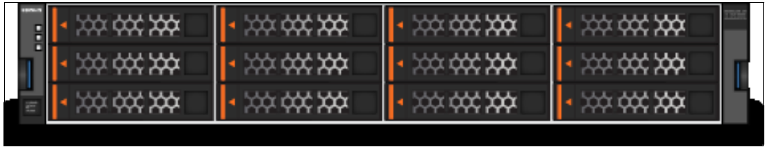
Figure 1-1 IBM Storwize V5000 front view for 2077/2078-12C and 12E enclosures
