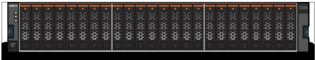
Figure 1-2 IBM Storwize V5000 front view for 2077/2078-24C and 24E enclosure
