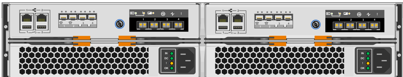
Figure 1-4 IBM Storwize V5000 controller rear view of models 12C and 24C
