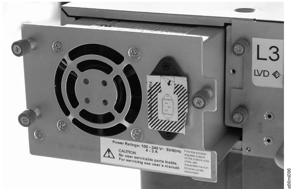
Figure 10-10. A power supply being removed from a 2U library
