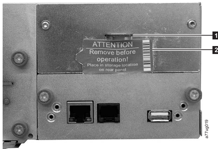
Figure 10-15. Library shipping lock and label storage location on the rear panel of the library
