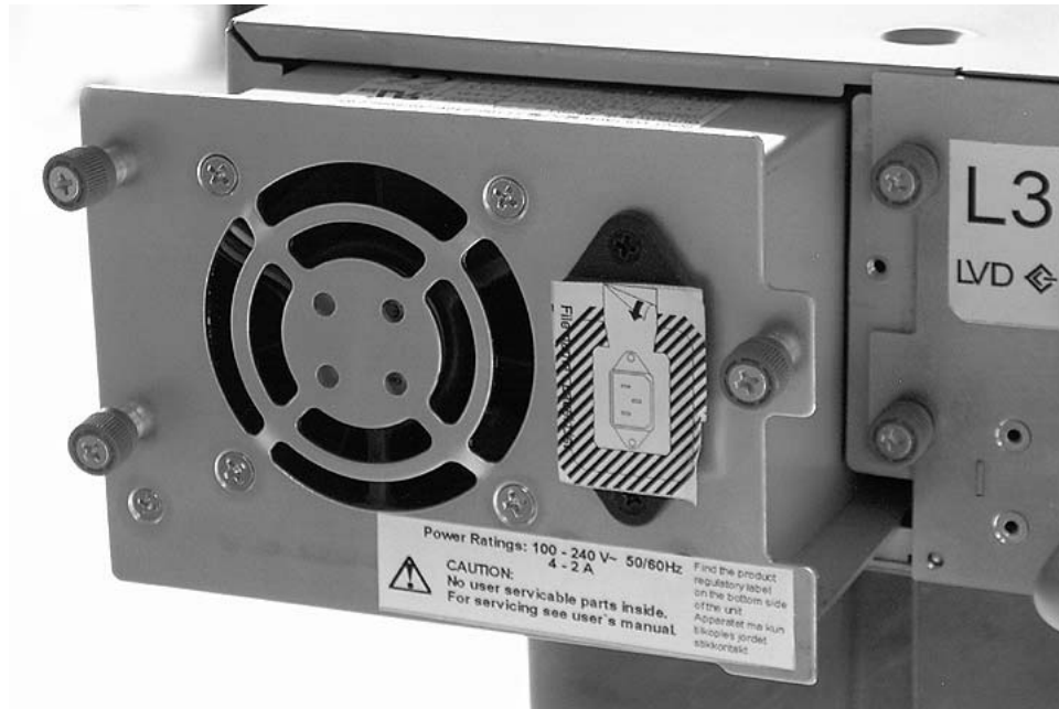
Figure 10-18. A power supply being removed from a library
