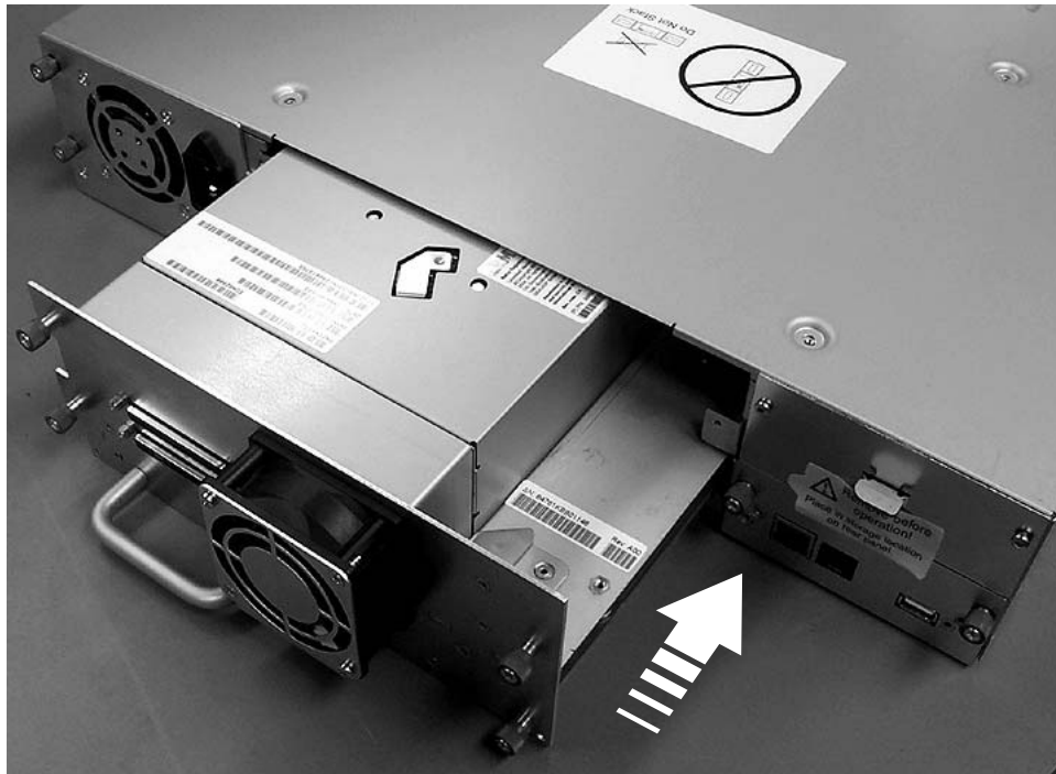
Figure 10-8. Pushing the drive sled into the library (drive sled without ESD springs shown)
