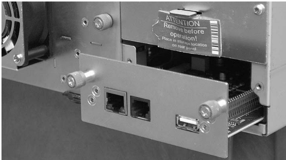
Figure 10-11. A Library Controller Card being removed from the library
