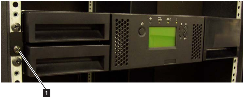
Figure 4-11. Securing the 2U library to the rack
