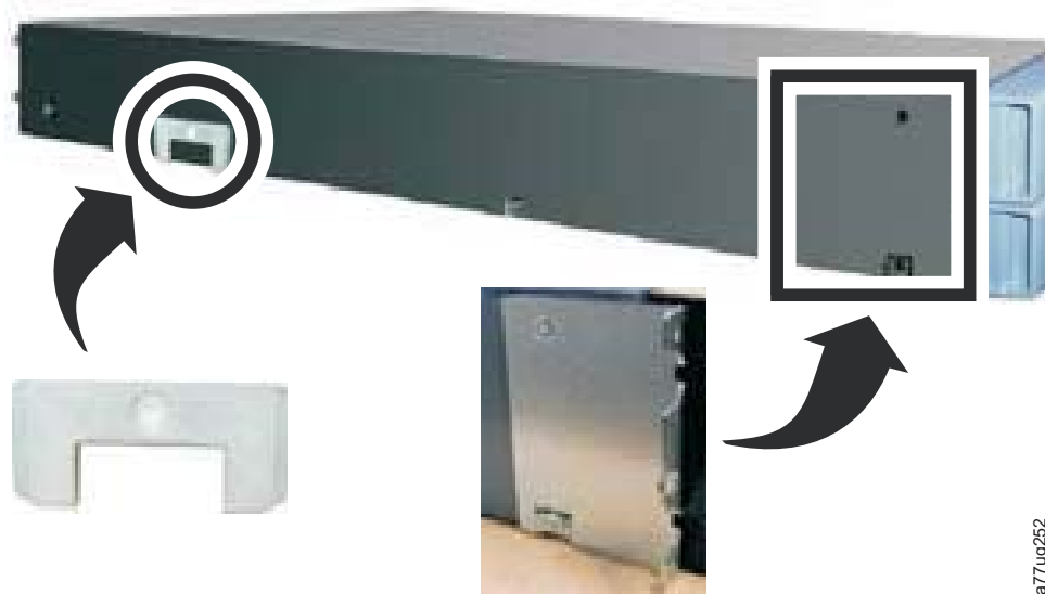
Figure 10-23. Mounting brackets and anchors for securing the library in a rack (one bracket and anchor on each side of the library)
