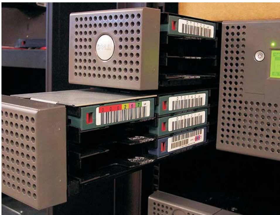
Figure 10-22. Left magazines pulled out of a 4U library (facing front of library)
