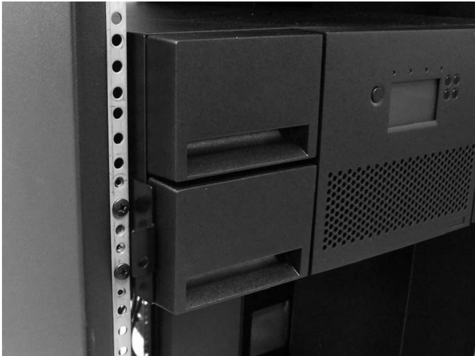
Figure 4-10. Sliding the 4U library into the rack
