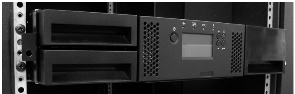
Figure 4-9. Sliding the 2U library into the rack
