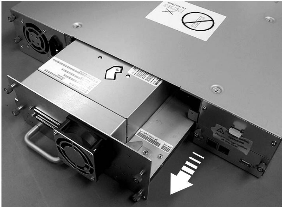
Figure 10-7. Pulling the drive sled out of the library (drive sled without ESD springs shown)
