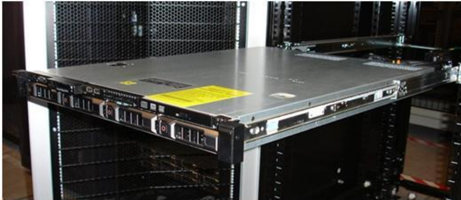
Figure 10. R415 Mounted in A3 Sliding Rails
