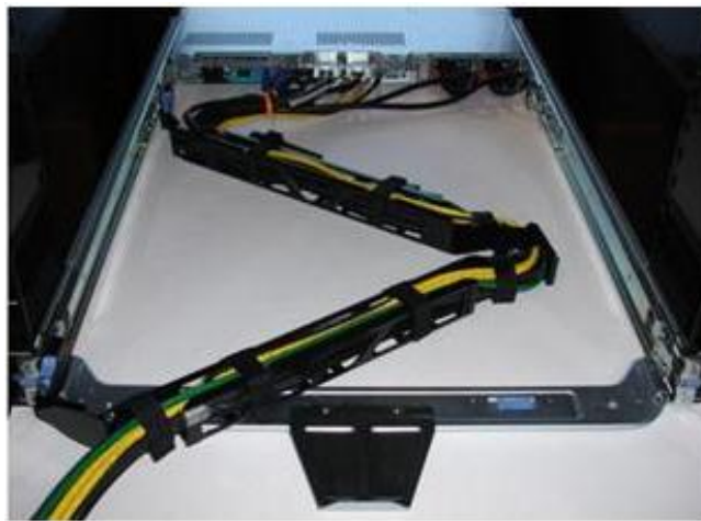
Figure 11. Back View of R415 Mounted in A3 Sliding Rails with CMA
