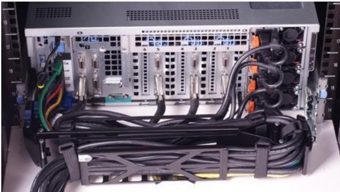
Figure 8. R910 CMA Mounted on the Side Opposite the Power Supplies (Recommended)
