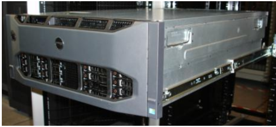
Figure 7. R910 Mounted in the B2 Sliding Rails
