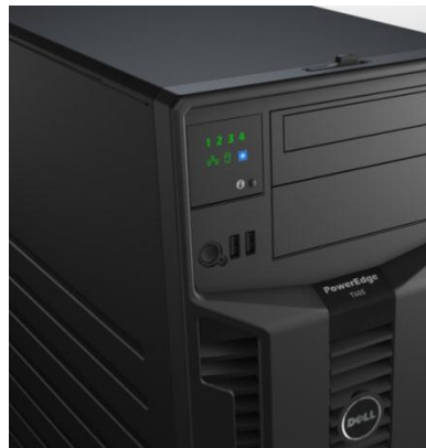
Figure 5. LED Control Panel
