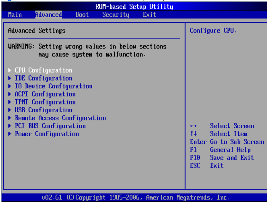
Figure 71 Advanced menu of the BIOS setup utility
