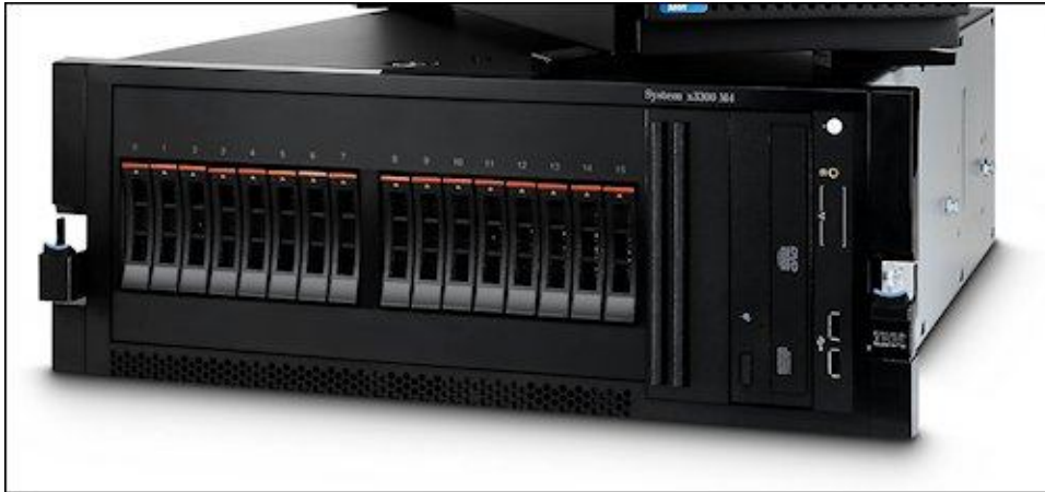
Figure 9. The IBM System x3300 M4 server with the Tower to Rack Conversion Kit
