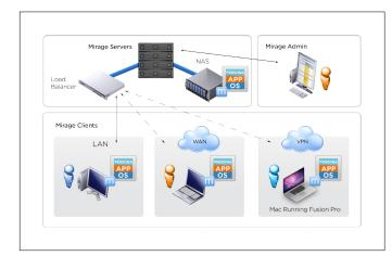
The Horizon Mirage architecture includes the Horizon Mirage server in the data center to centralize desktop management and protection, the Horizon Mirage client to create a local cache for an optimal user experience at the endpoint, and advanced WAN optimization technology to speed bidirectional synchronization over the WAN.
